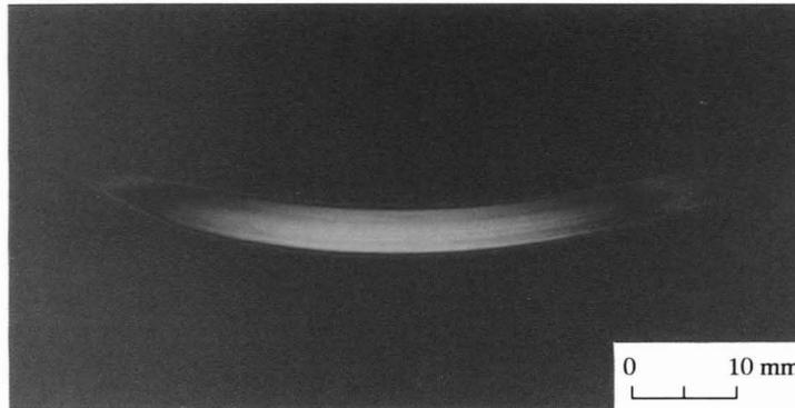
(a) Photo of the crescent blue beam radiated from the channel waveguide Cerenkov SHG element, taken from a white paper plate.
