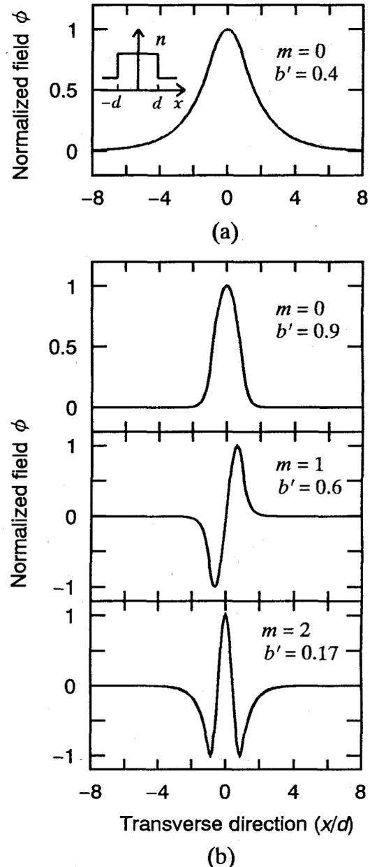
Fig. 1 Mode field distributions obtained by the numerical (dotted curves) and analytical methods (solid curves) with step index profile; (a) narrow waveguide and (b) wide waveguide.
