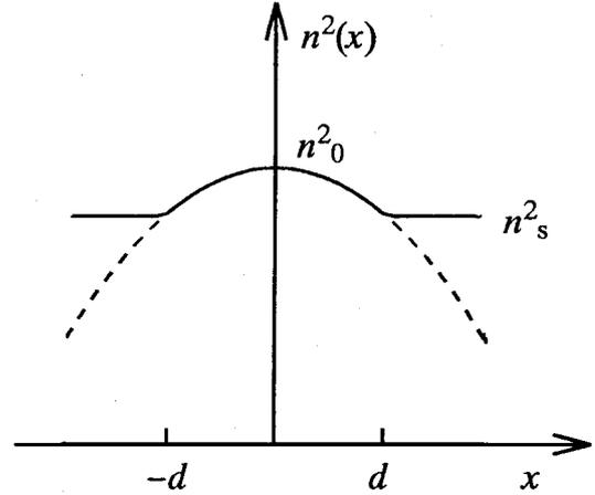
Fig. 2 The truncated square index distribution shown by the solid curve for which the present calculation is done and the typical infinite square index profile shown by the dashed curve.
