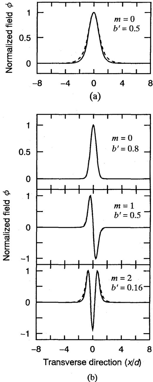
Fig. 3 Mode field distributions for the truncated square index profile obtained by the numerical (dotted curves) and analytical calculations (solid curves); (a) single-mode waveguide and (b) multi-mode waveguide.
