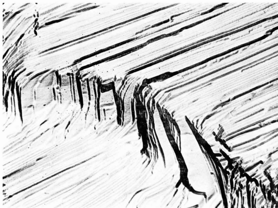
Fig. 4 Electron micrograph of fracture surface of the plate-like crystal. \times 25000
