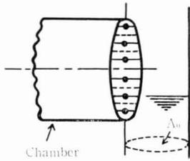
Fig. 13 Chamber divided into several sections at given levels.
