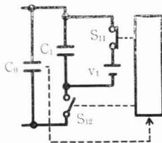
Fig. 9 Analog circuit for varying cross-sectional surge tank.
