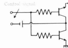
Fig. 2 Transistor switch for direct analog simulator.
