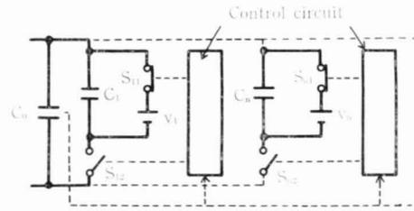
Fig. 1 Circuit which insert or remove additional capacitors.
