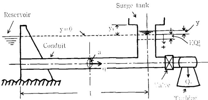
Fig. 5 Oscillatory system with varying cross-sectional surge tank.
