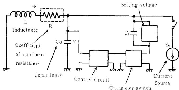
Fig. 6 Analog circuit for oscillatory system with varying cross-sectional surge tank.
