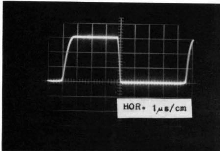
Fig. 3 Time-response of transistor switch.
