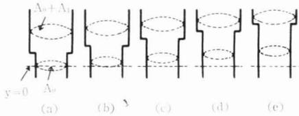
Fig. 7 Varying cross-sectional surge tanks.
