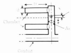
Fig. 12 Chamber surge tank system.
