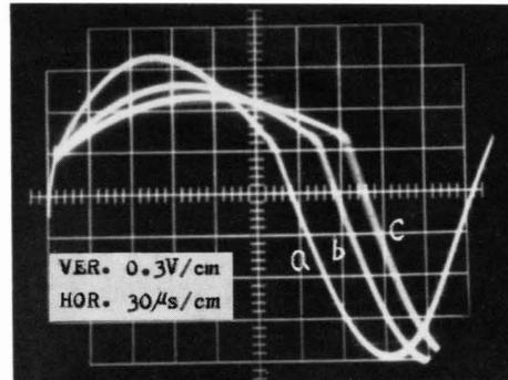
Fig. 11 Oscillograms of voltage corresponded to variation of water level in surge tank.
