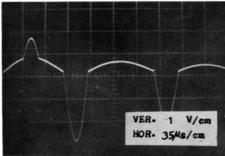
Fig. 14 Oscillograms of voltage corresponded to variation of water level in chamber surge tank.
