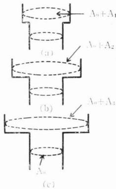
Fig. 8 Varying cross-sectional surge tanks.
