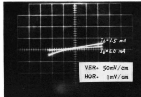
Fig. 4 Dynamic characteristics of transistor switch.
