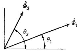
Fig.1 Vector representative method for distorted wave on the vector-plane (The figure shows an example consisting of the fundamental and the third harmonics).
