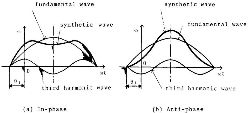
Fig.2 Diagrams illustrating "in-phase" and "anti-phase".
