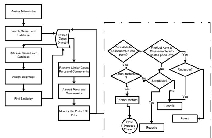
Figure 1. Computer aided remanufacturing evaluation system (CARES) simulation method.
