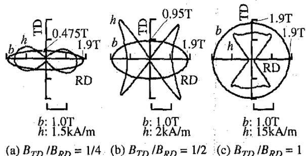
Fig. 8. Loci of flux density and magnetic field strength under rotating flux condition (JIS 35G165,  $f=50$ Hz, DET).
