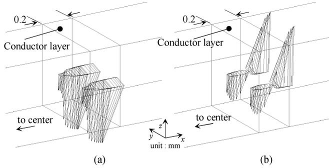
Fig. 5. AC current distributions in conductor layer at model I ( $n$  value = 8,  $L_p = 300$ ). (a)  $\omega t = -\pi/2$  ( $|J_{\max}| = 4.37 \times 10^7$  A/m<sup>2</sup>). (b)  $\omega t = 0$  ( $|J_{\max}| = 4.14 \times 10^7$  A/m<sup>2</sup>).
