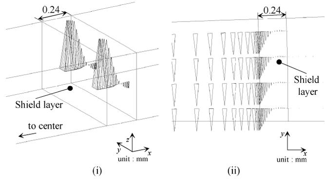
Fig. 6. Flux and current distributions in a shield layer of model I (model I: 40 HTS tape wire without interval between wires in a shield layer,  $d = 0$  mm, at  $\omega t = -\pi/2$ ,  $n$  value = 8). (i) Current distribution in a shield layer; (ii) flux distribution around a shield layer.
