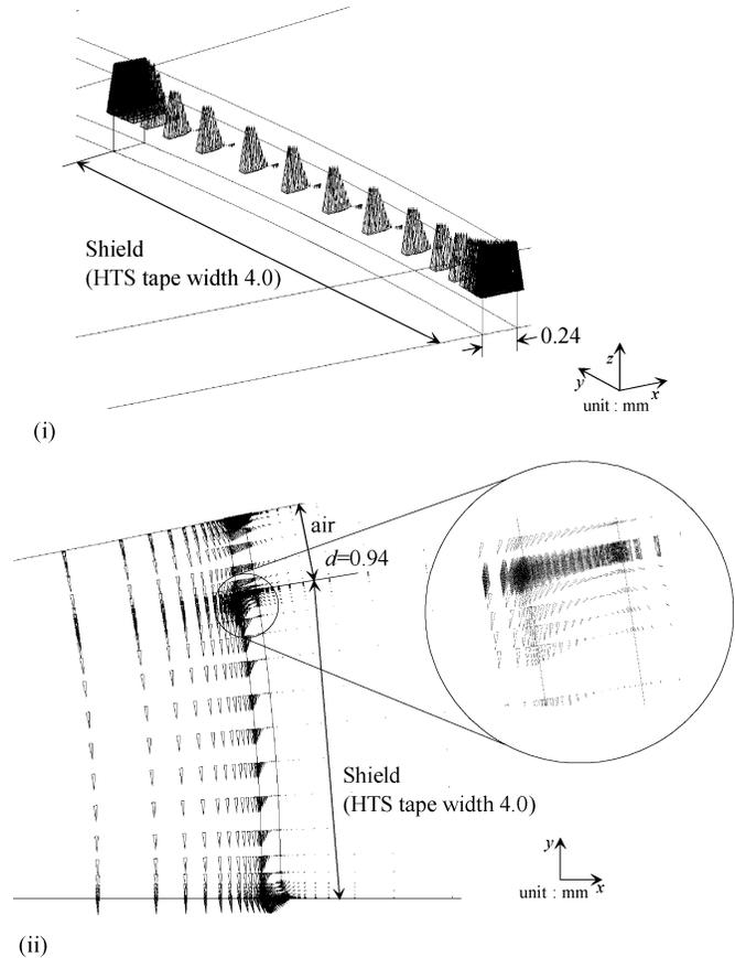
Fig. 7. Flux and current distributions in a shield layer of model II (model II: 32 HTS tape wires in a shield layer,  $d = 0.94$  mm, at  $\omega t = -\pi/2$ ,  $n$  value = 8). (i) Current distribution in a shield layer; (ii) flux distribution around a shield layer.
