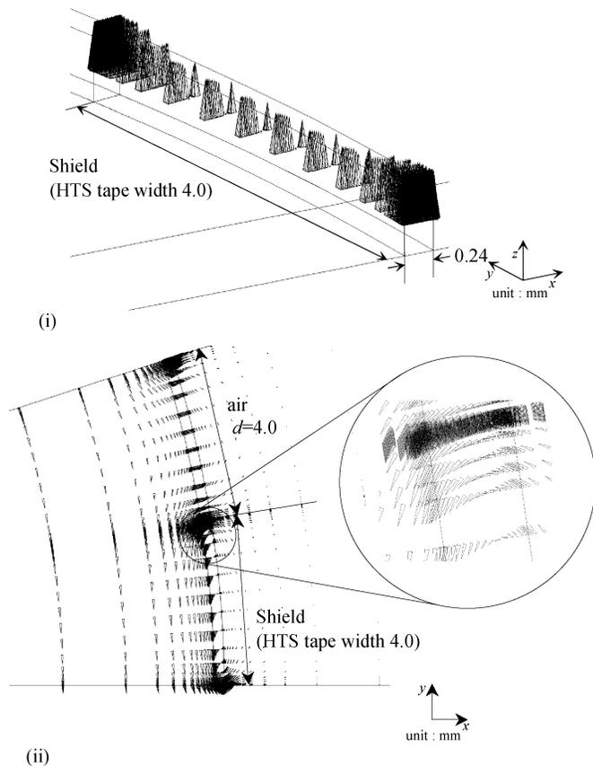
Fig. 8. Flux and current distributions in a shield layer of model III (model III : 20 HTS tape wires in a shield layer,  $d = 4.0$  mm, at  $\omega t = -\pi/2$ ,  $n$  value = 8). (i) Current distribution in a shield layer; (ii) flux distribution around a shield layer.
