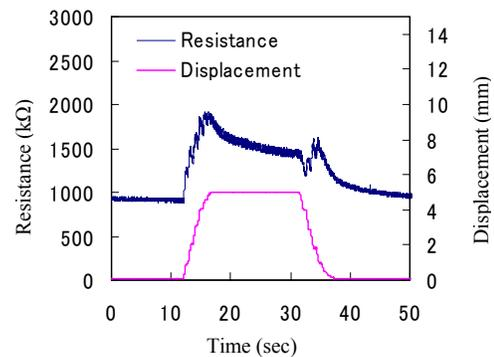
Fig.5 Relationship between displacement and electrical resistance of type-C
