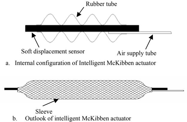
Fig.8 Configuration of Intelligent McKibben actuator
