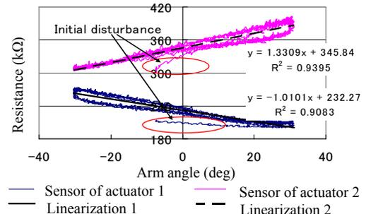
Fig.15 Dynamic characteristics of sensor 1 and sensor 2
