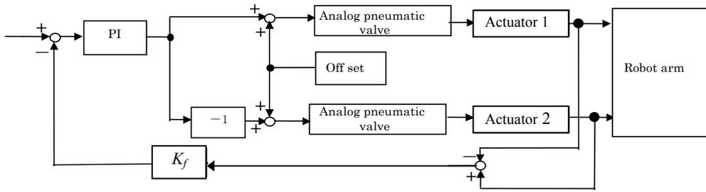
Fig.17 Servo control system of robot arm mechanism
