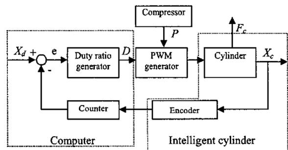
Figure 11. Control system of intelligent cylinder
