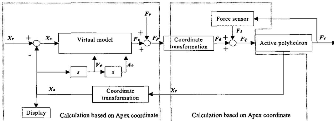
Figure 14. Block diagram of driver program
