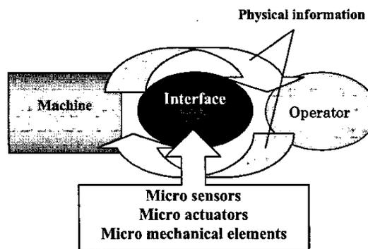
Figure 1. Physical man-machine (PMI)
