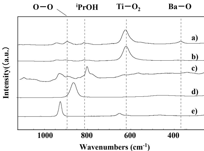
Fig. 2. Raman Spectra of the precursor solutions; a) BaTi precursor solution ( $\text{Ba}(\text{CH}_3\text{COO})_2 + \text{Ti citric acid} + \text{H}_2\text{O}_2$ ), b) Ti citric acid +  $\text{H}_2\text{O}_2$ , c) Ti citric acid, d)  $\text{H}_2\text{O}_2$  and e)  $\text{Ba}(\text{CH}_3\text{COO})_2$ .
