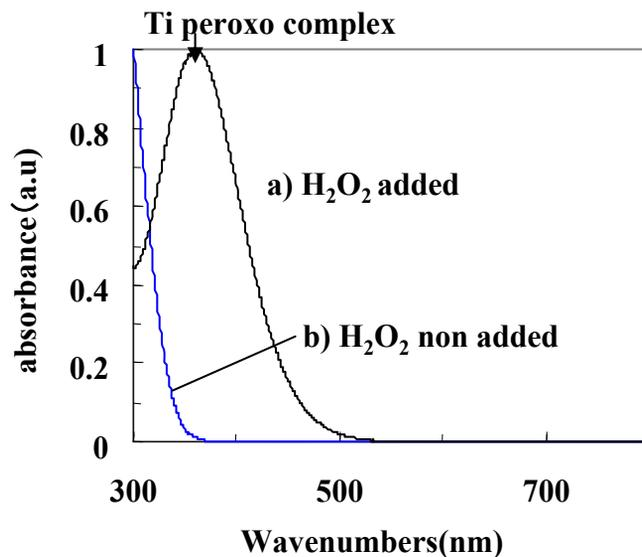
Fig. 1. UV-vis spectra of Ba-Ti precursor solutions.
