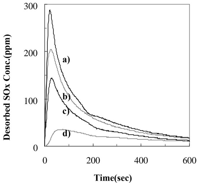
**Fig. 8.** Sulfur desorption profiles during  $\text{SO}_x$  regeneration from NSR catalysts; a) BaTi-B at  $650^\circ\text{C}$ , b) BaTi-B at  $600^\circ\text{C}$ , c) Ba-B at  $650^\circ\text{C}$  and d) Ba-B at  $600^\circ\text{C}$ .
