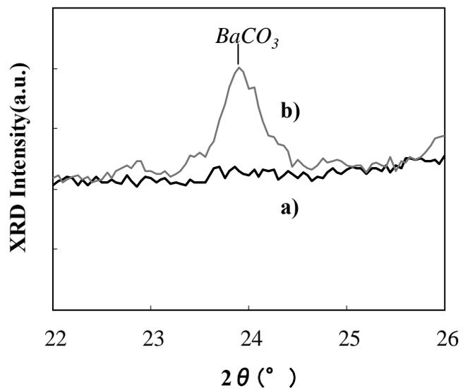
**Fig.5.** XRD patterns of fresh catalysts; a) BaTi-A and b) Ba-A.
