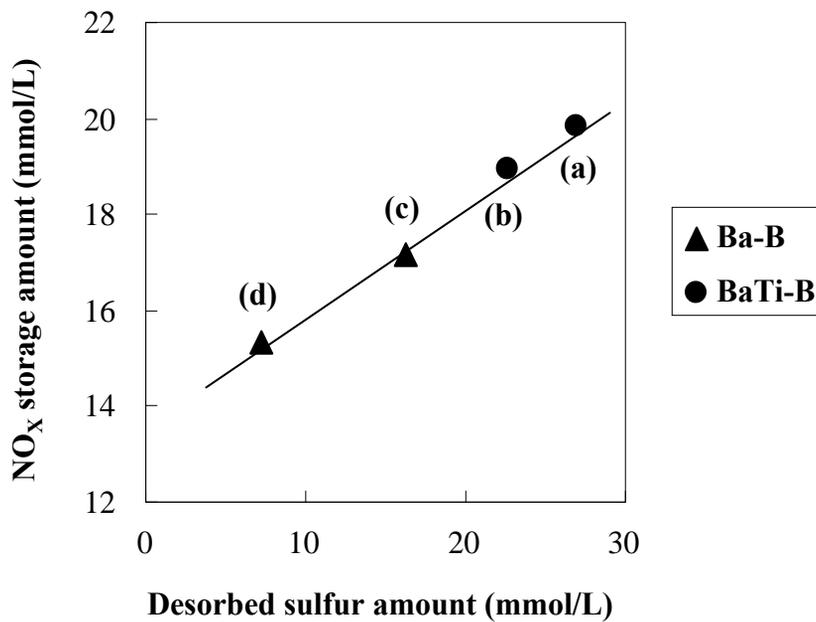
**Fig. 11.** The relationship between desorbed sulfur and NO<sub>x</sub> storage amounts after sulfur regeneration at 600°C or 650°C; a) BaTi-B at 650°C, b) BaTi-B at 600 °C, c) Ba-B at 650°C and d) Ba-B at 600°C.
