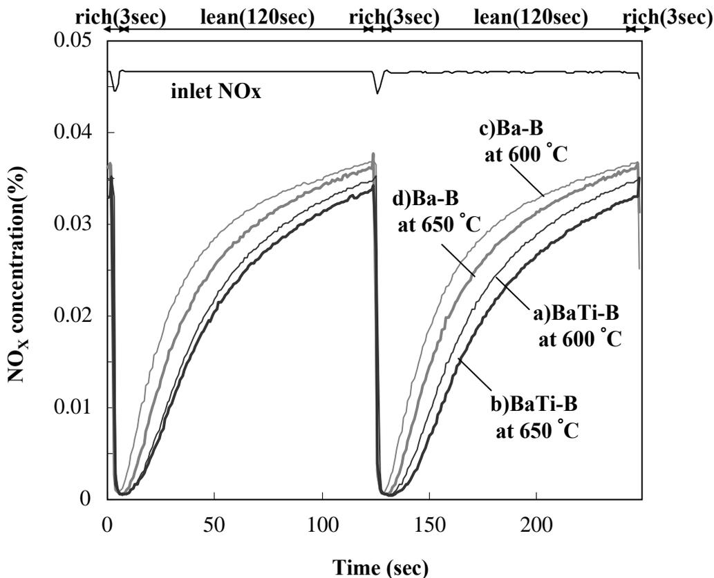
Fig. 9. NO<sub>x</sub> concentration profiles at 400°C during lean/rich cycle test over BaTi-B and Ba-B after the sulfur desorption procedure at 600 and 650°C.
