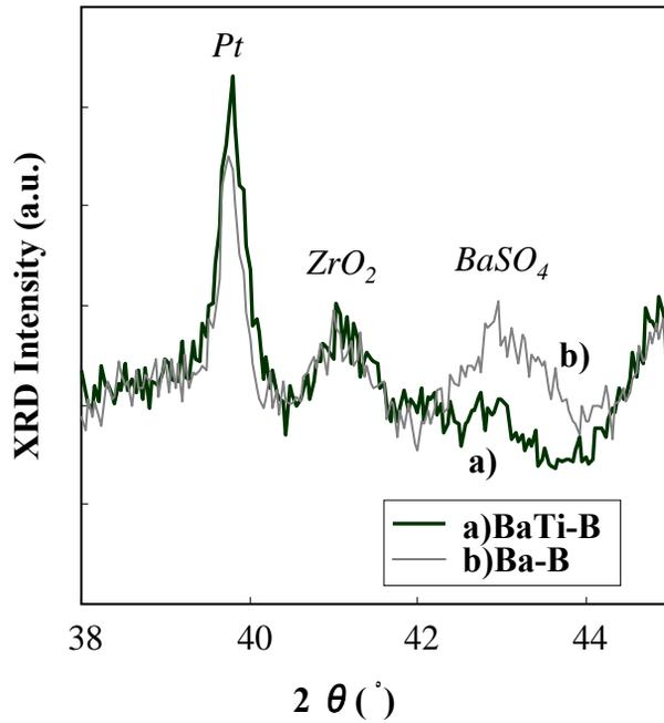
**Fig. 7.** XRD patterns of catalysts after sulfur aging; a)BaTi-B and b)Ba-B.
