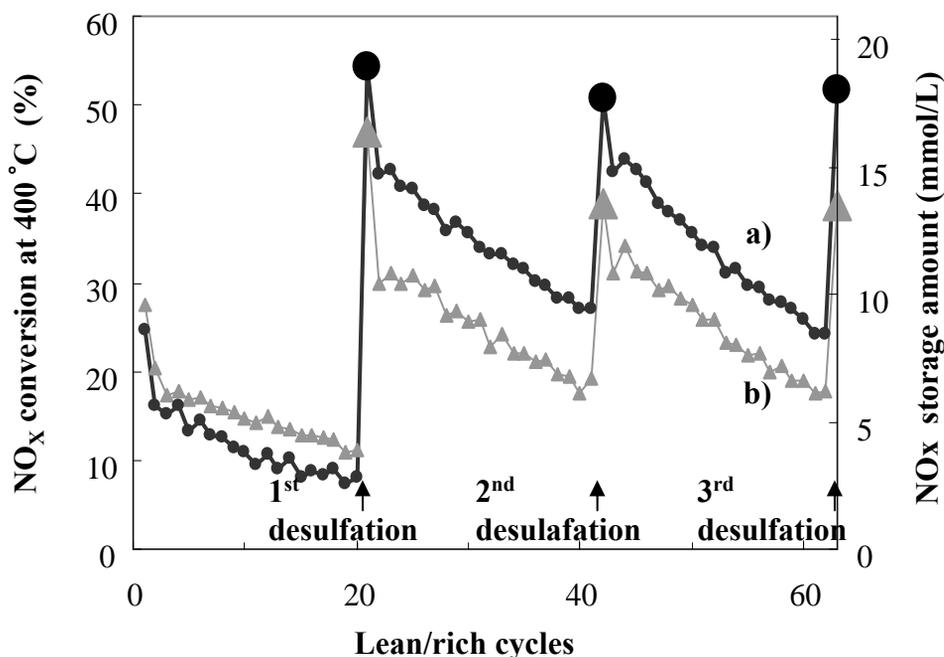
Fig. 10. NO<sub>x</sub> conversion change at 400°C during repetitive procedures (20 lean/rich cycles at 400°C) and desorption (rich at 650°C) over a) BaTi-B and b) Ba-B catalysts.
