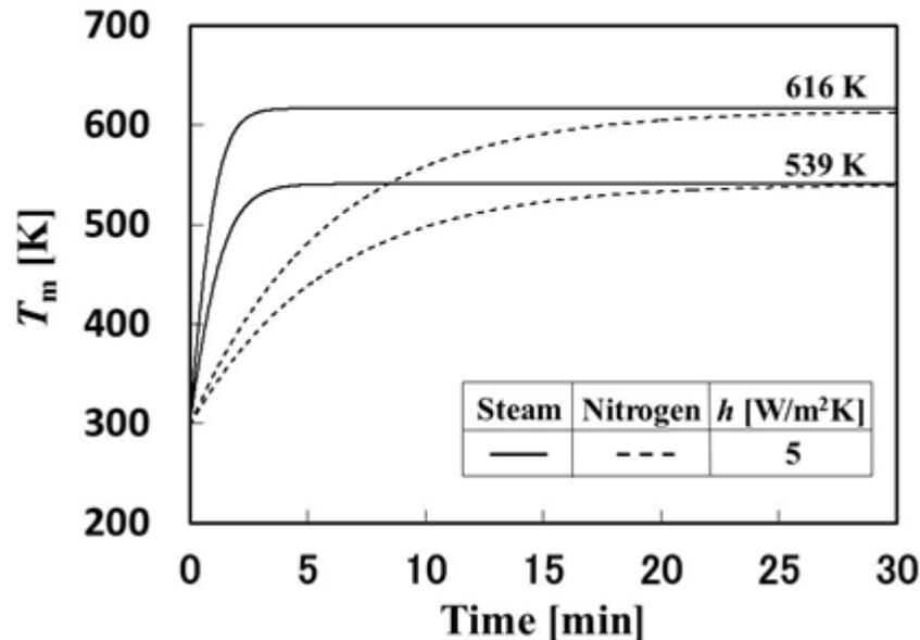
**Fig. 1** Comparison of temporal change in calculated temperature change between superheated steam and nitrogen gas at the same carbonization temperature.
