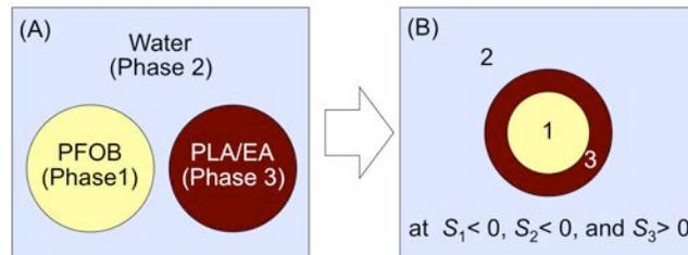
Figure 2 (A) Designation of each phase to calculate spreading coefficients. (B) Expected equilibrium core-shell configuration obtained at  $S_1 < 0, S_2 < 0, \text{ and } S_3 > 0$ .
